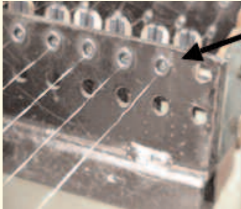
Ceramic guide eye insert into grounded steel holder
