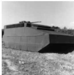
The CAV-ATD replaces traditional all-metallic tracked vehicle chassis with one built of S-2 Glass reinforced composites.
