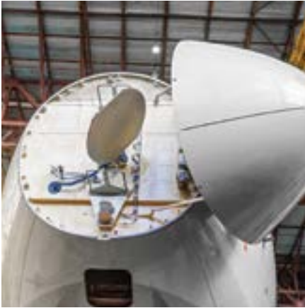
Radar Transparency Delivers 20% lower dielectric constant than conventional E-Glass fiber.
